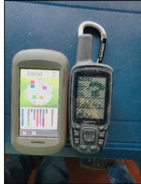
Image 3. Verification in the measurement of geographic coordinates from the two equipment to be used in the field. A new GPS is used as a reference.
